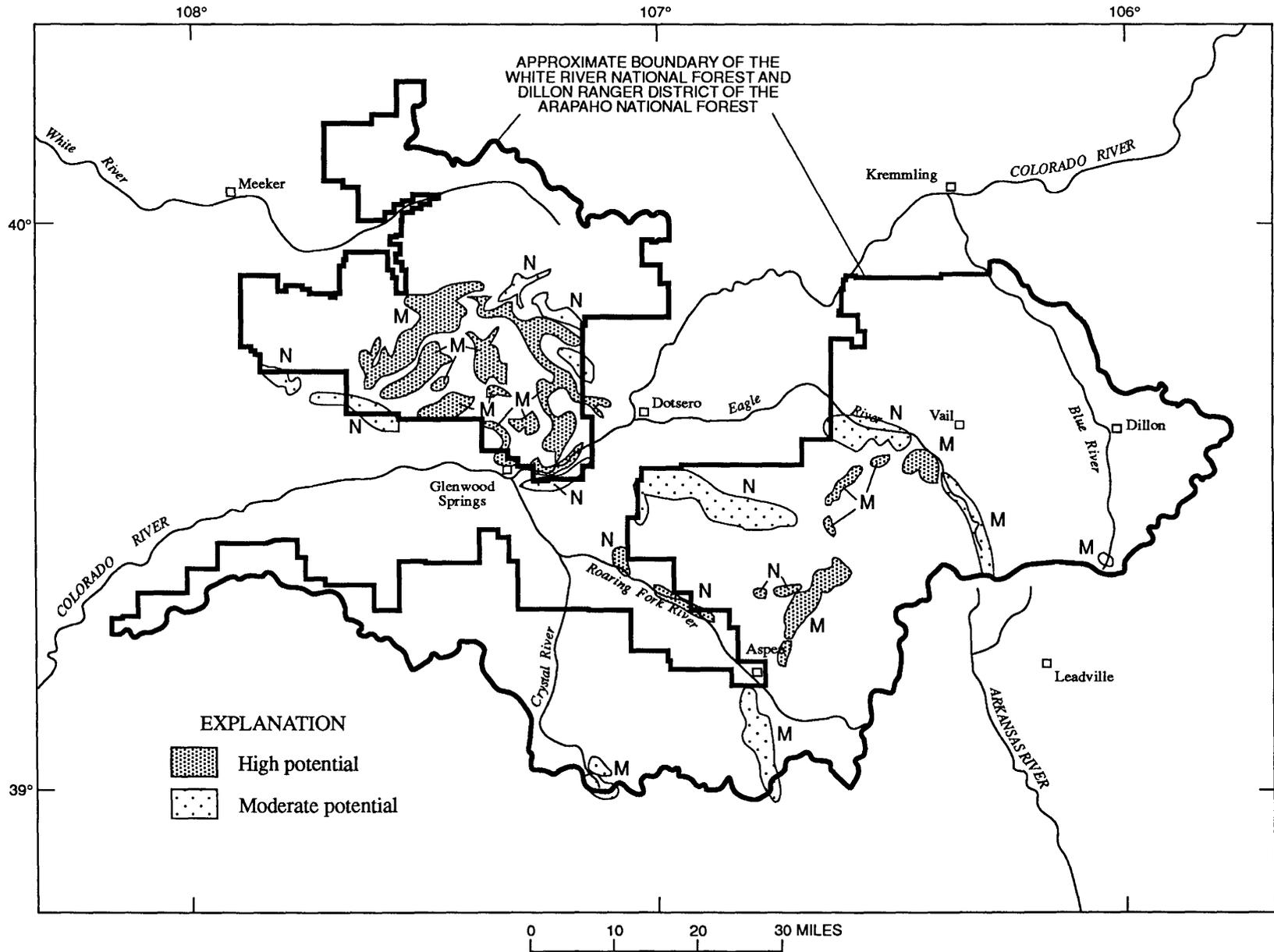
**Figure 9.** Mineral resource potential map for high-calcium limestone (deposit type M) and gypsum in evaporite deposits (deposit type N) in the White River National Forest and Dillon Ranger District of the Arapaho National Forest, Colorado. Where areas of different potential overlap, only the area of high potential is shown.
