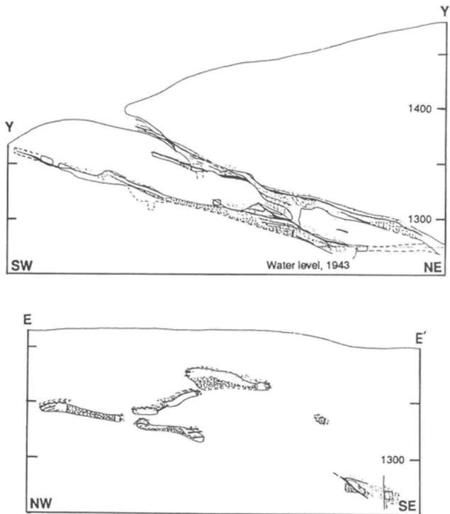
**Figure 6.** Mine section drawings from White and Eric (1944, pl. 6). Heavy black is “massive sulfide including schist with abundant disseminated sulfide”; light dashed lines are foliation. Displacement sense shown on small vertical fault. Adits, stopes, mine rubble indicated. E-E’, Y-Y’ located on figure 5. Numbers on vertical axes indicate elevation.
