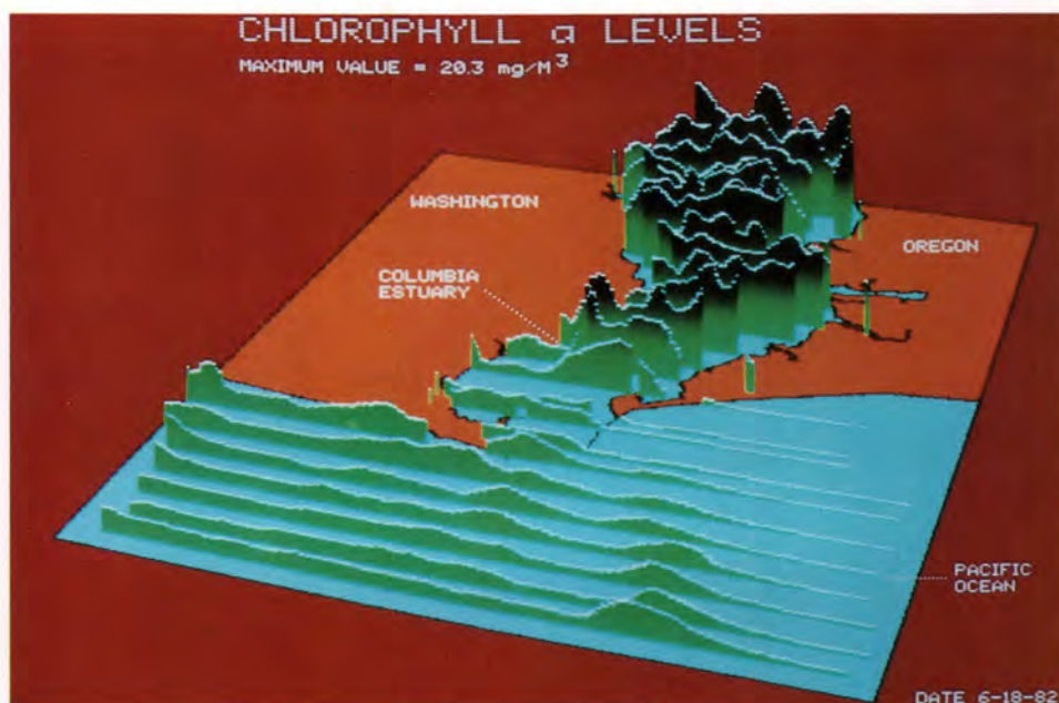
Figure 14. Laser fluorescence data from the Columbia River estuary, Washington, showing chlorophyll concentrations in the water. Courtesy of the Environmental Protection Agency, Las Vegas, Nev.
