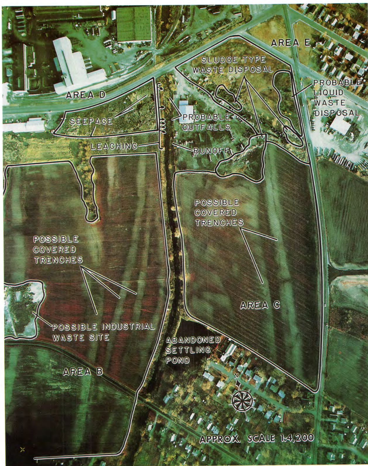
Figure 12. Color-infrared aerial photograph of a potential industrial pollution site. Photograph courtesy of the Environmental Protection Agency, Las Vegas, Nev., acquired December 18, 1980.
