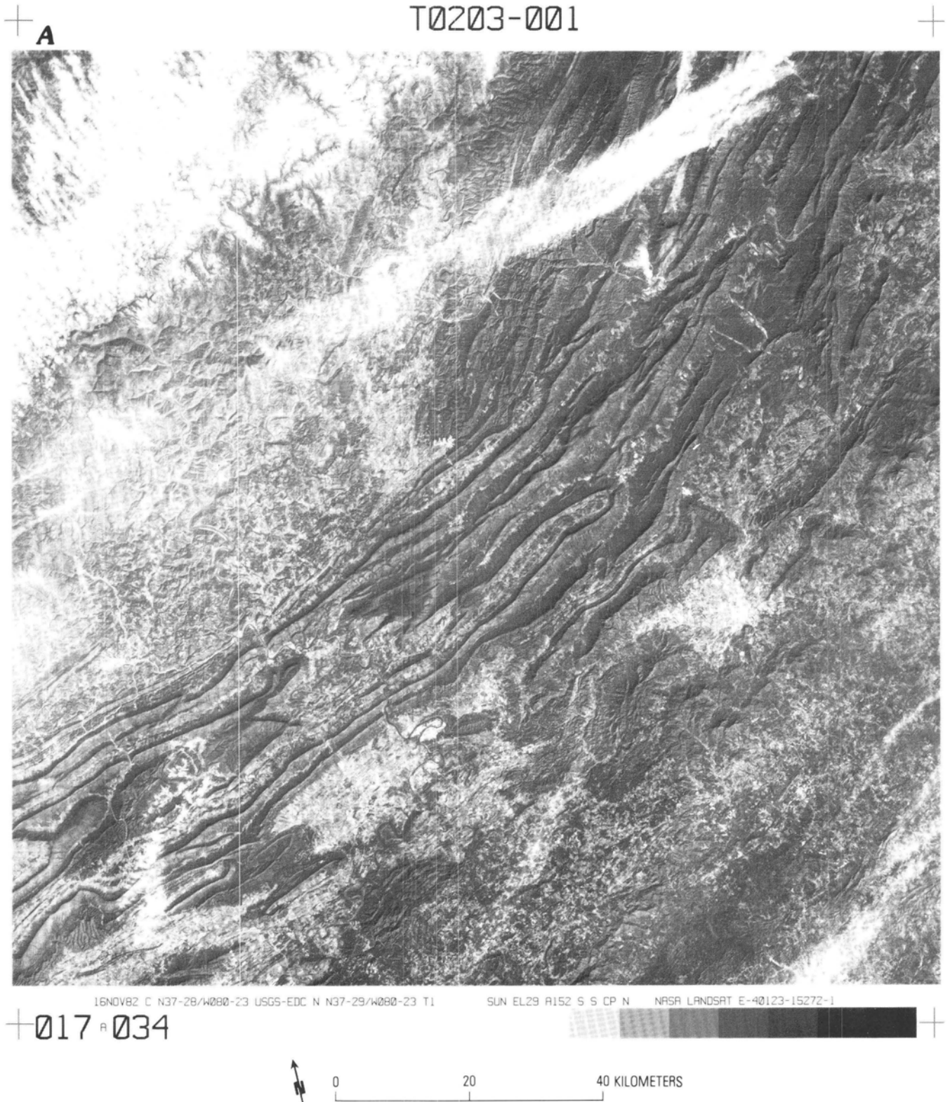
Figure 3. Landsat 4 thematic mapper (TM) images (ID 40123-15272, path 17, row 34) acquired November 16, 1982, over the folded and faulted Appalachian Mountains near Roanoke, Virginia (right-center of image). The narrow spectral bands and 30-m resolution of the TM provide significant improvement over the multispectral scanner. From the lower right
