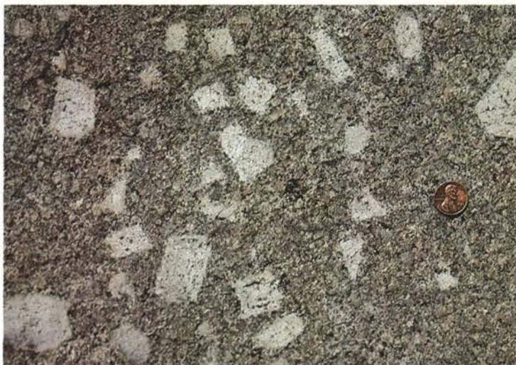
PORPHYRYTIC TEXTURE in Cathedral Peak Granodiorite, with potassium feldspar phenocrysts much larger than the other minerals in the rock matrix. (Fig. 14)
