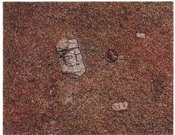
JOHNSON GRANITE PORPHYRY, showing potassium feldspar phenocrysts set in a fine-grained matrix. (Fig. 21)
