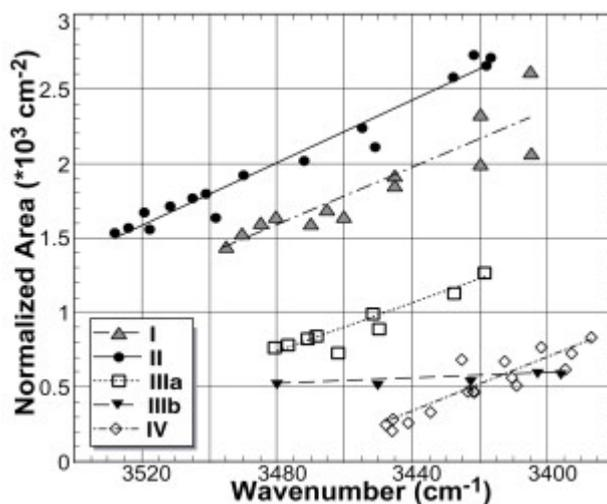
**Figure 11** : Plot diagram showing band area converted to normalized areas for a sample thickness of 1 cm, as a function of the peak top position (wavenumber). Slopes of regression lines are close to  $-9$  for all types of inclusions, except for FI IIIb in sample III.
