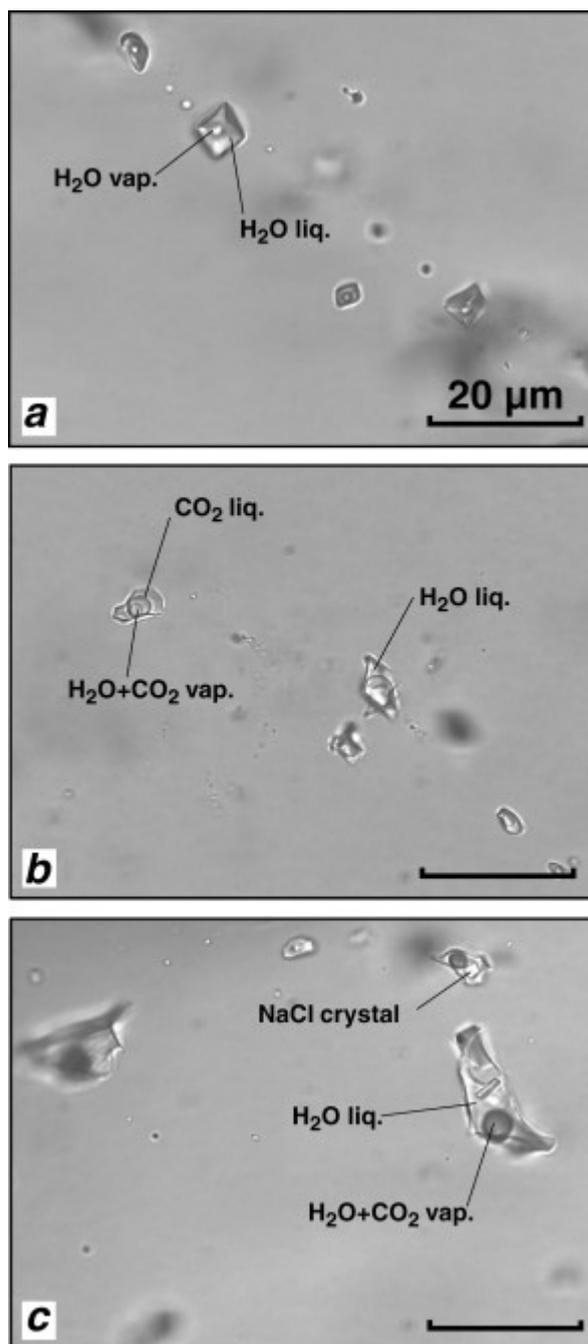
**Figure 2** : High magnification photomicrographs of typical fluid-inclusions encountered in the studied samples. a) Secondary biphased  $\text{H}_2\text{O}$ - $\text{NaCl}$  inclusions planes, with low to moderate salinity and high filling ratios (FI I, II, IIIa). b) Secondary triphased  $\text{H}_2\text{O}$ - $\text{NaCl}$ - $\text{CO}_2$  inclusions planes (FI IIIb). c) Biphased salts- $\text{CO}_2$  inclusions clusters (FI IV).
