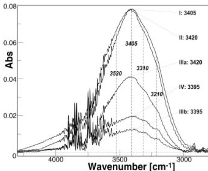
**Figure 5 :** IR spectra of fluid inclusions at room temperature, with positions of shoulder components at 3210, 3310, 3405 and 3520  $\text{cm}^{-1}$  in a normalized absorbance-versus-wavenumber diagram. All the spectra are shown after baseline correction and normalized to a thickness of 1 cm. Apparent peak positions of FI I, II, IIIa, IIIb and IV are at 3405, 3420, 3420, 3395 and 3395  $\text{cm}^{-1}$ , respectively.
