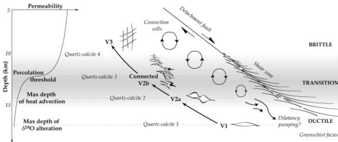
**Figure 12 :** Synthetic diagram showing the simultaneous evolutions of veining, quartz-calcite precipitation, fracture permeability and fluid movement as the footwall of the shear zone enters the brittle regime during exhumation (not to scale). The appearance of an interconnected V2b vein network in late ductile context is interpreted as the mechanism responsible for fluid circulation increase ("percolation threshold") recorded by oxygen isotopes in quartz-calcite 3.
