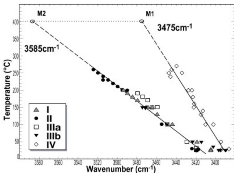
**Figure 12 :** Plot diagram of apparent peak positions of IR OH bands as a function of temperature for all fluid inclusions. FI I, II, IIIa and IIIb show linear trends with a mean slope of 0.50, which reaches 3585 cm<sup>-1</sup> by extrapolation to 400 °C. FI IV show another linear trend with a slope of 0.25, attaining 3475 cm<sup>-1</sup> by extrapolation to 400 °C.
