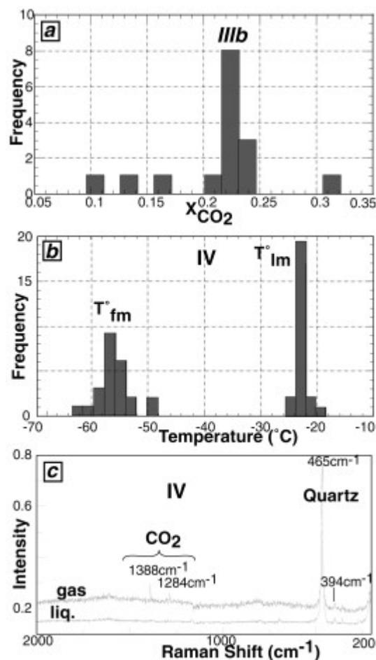
**Figure 4** : Frequency histograms and Raman shift of FI IIIb triphased fluid-inclusions (sample III) and FI IV salts-CO<sub>2</sub> inclusions (sample IV). a) X<sub>CO<sub>2</sub></sub> in FI IIIb centered on 0.23. b) First and last melting temperatures (T<sub>fm</sub> and T<sub>lm</sub>, respectively) in FI IV are centered around -55 and -24 °C, respectively. c) Raman spectra of the vapor phase in FI IV, showing the two sharp peaks of gaseous CO<sub>2</sub> at 1284 and 1388 cm<sup>-1</sup>.
