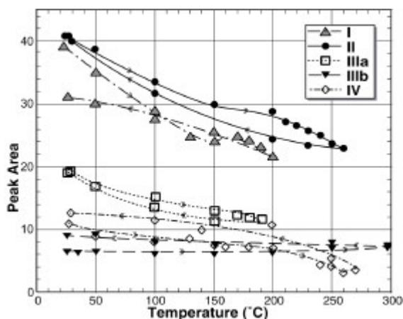
Figure 8 : Plot diagrams showing peak area (after baseline correction) as a function of temperature, upon heating and cooling. Band area is recovered at room temperature, except for FI I, which show a lost of 20 % band area.
