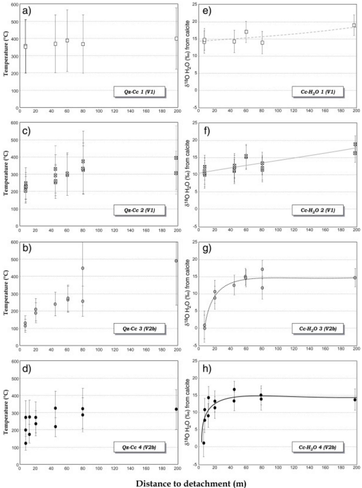
**Figure 9 :** Temperatures calculated from quartz-calcite fractionation (a; b; c; d), and oxygen isotope composition of water in equilibrium with calcite at these temperatures (e; f; g; h), as a function of distance to detachment (Qz-Cc and Cc-H<sub>2</sub>O calibrations from Sharp & Kirschner, 1994 & Zheng, 1999, respectively). a); e) Generation 1 quartz-calcite pairs in V1 veins. b); f) Generation 2 in V1. c); g) Generation 3, V2b veins. d); h) Generation 4 in V2b. Error bars 1  $\sigma$ .
