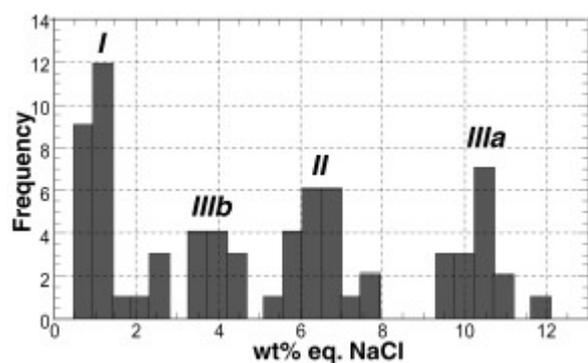
**Figure 3** : Frequency histograms of salinities encountered in H<sub>2</sub>O-NaCl fluid-inclusions. a) Peak frequency in FI I (sample I) is centered on 1 %wt eq. NaCl. b) Sample II fluid-inclusion salinities are centered on 6.4 %wt eq. NaCl (FI II). c) Salinity in FI IIIa H<sub>2</sub>O-NaCl inclusions (sample III) range between 10 and 10.5 %wt eq. NaCl.
