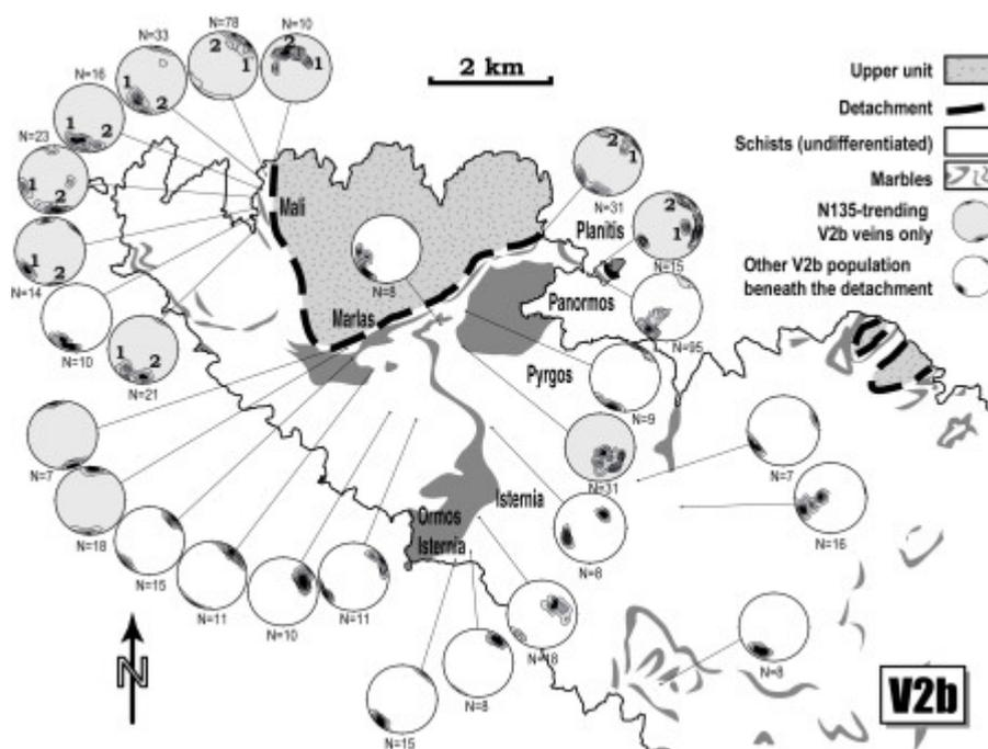
**Figure 4 :** Stereograms of poles of V2b veins on the north of Tinos (corrected from the dip of foliation, equal area, lower hemisphere). Empty stereograms: N135°E-trending V2b. Grey stereograms: V2b rotation in the vicinity of the detachment. The main N135°E direction is split into two separate families at Planitis. Progressive rotation from N135 to N80°E azimuth toward the detachment of Marlas. Two distinct directions of V2b under the detachment of Mali, oriented N135°E and N80 to N100°E.
