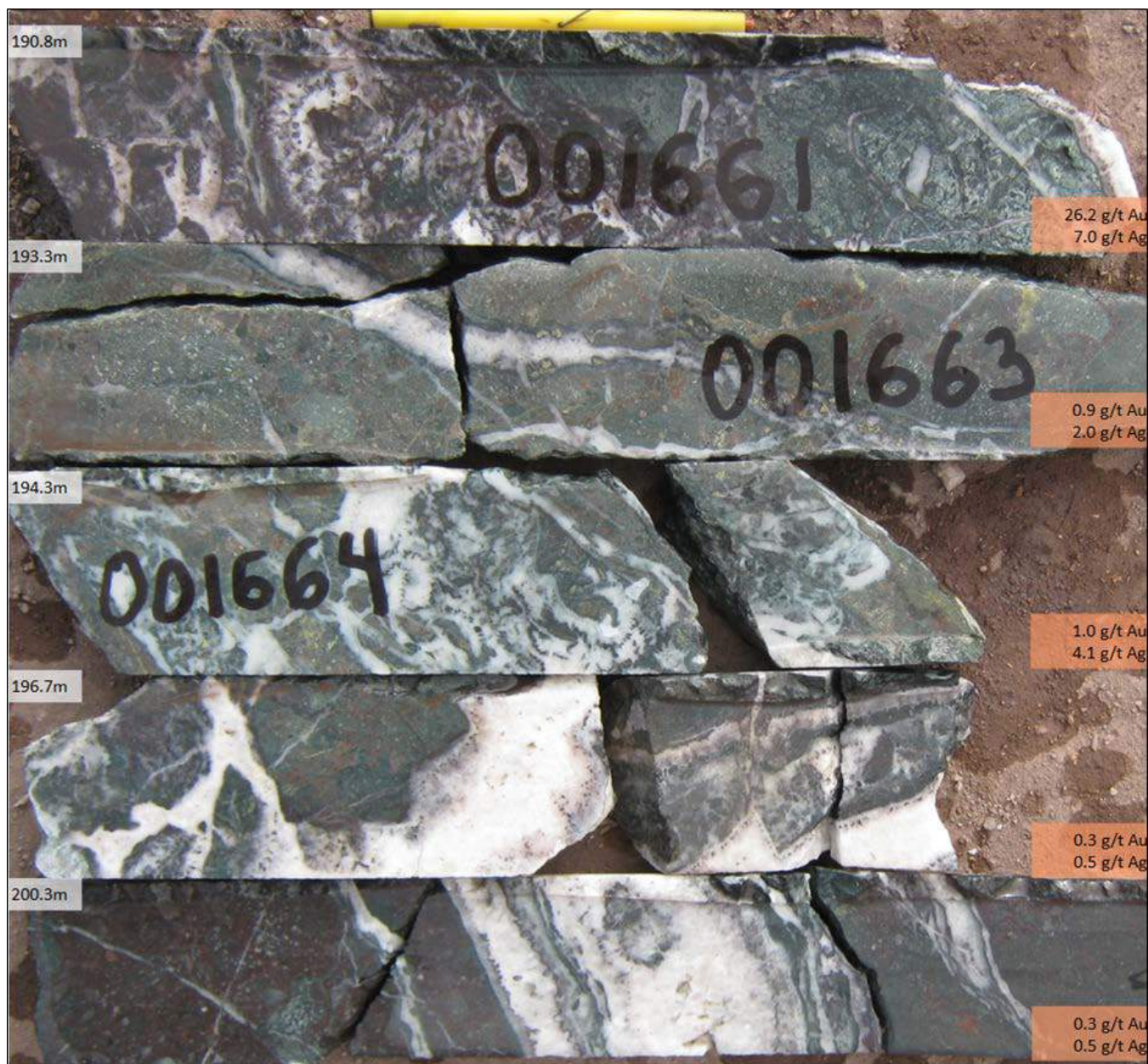
Mineralized Quartz-Galena-Sphalerite_Pyrite_Hematite Veins and Adjacent Hematitic Breccia Zone in Footwall
