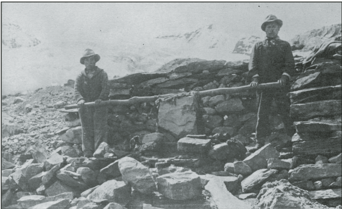
Figure 2. Manual stone mill, or quimbalete , used to crush gold-bearing quartz at Rinconada San Francisco, elevation of more than 5000 m, extreme northwest of Nevado Ananea, Prov. Sandia, Dept. Puno. (Photograph by G. Petersen G., 30 April 1945.)
