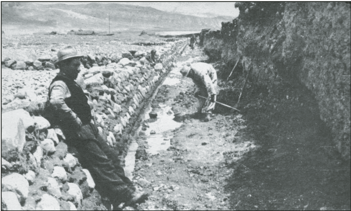
Figure 5. Alluvial gold prospecting at Pampa Blanca, Prov. Sandia, Dept. Puno, elevation of 4800 m. To the right are the gravels that comprise the alluvial gold occurrence and the gold is washed in the canal using glacial meltwater that comes from Nevado Ananea (5835 m). In the distance to the left is Pampa Blanca and in the center is Laguna Sillacunca, which supplies water to the artisanal gold miners at Poto. (Photograph by G. Petersen G., 29 March 1945.)
