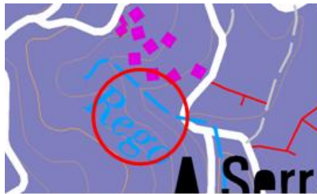
Figure 4: Linear text too distant to the line feature (Error type 01)
