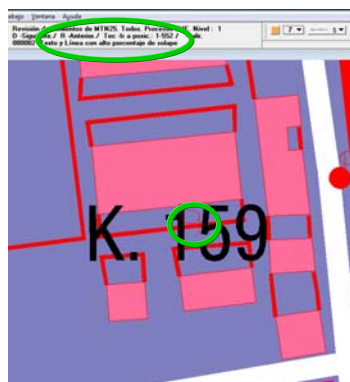
Figure 12: Text and line overlapping error review (Error type 02)
