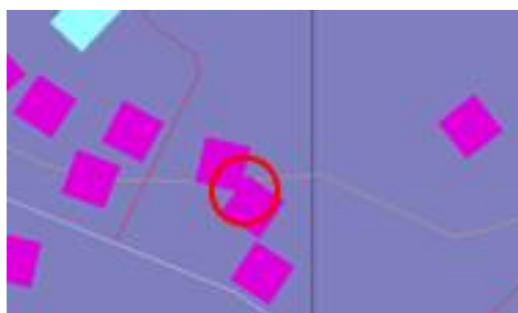
Figure 5: Two buildings overlapping (Error type 02)
