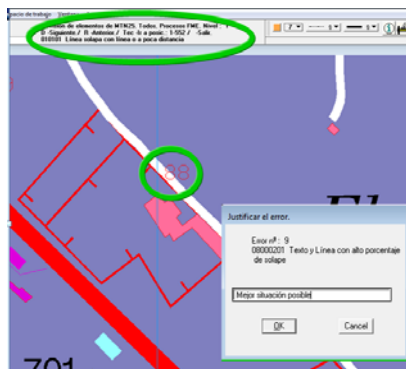
Figure 15. Justification of error of Line-Line overlapping (Error type 02)
