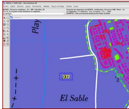
Figure 16: Justified error due to distance between bounded-text and bounded-point
