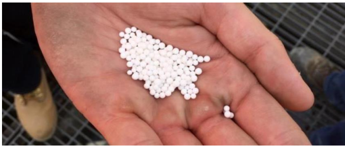
Figure 2.13 Grinding media used in stirred mills
