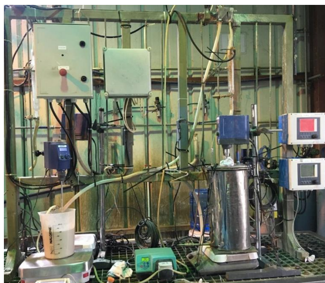
Figure 3.2 Arrangement of equipment and instruments for the atmospheric leaching test at the Envirogold facility in the Dominican Republic.
