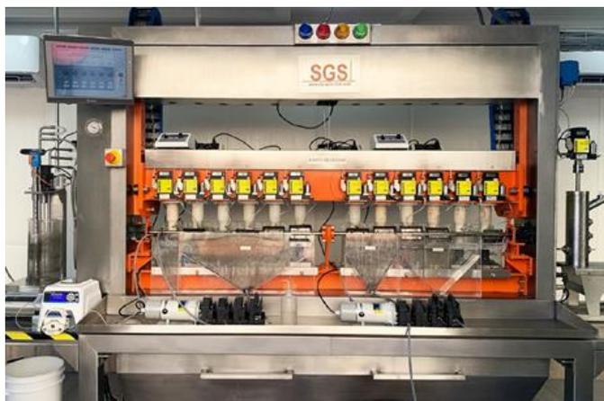
Figure 1: SGS Mini Pilot Plant (MPP), flotation units.
