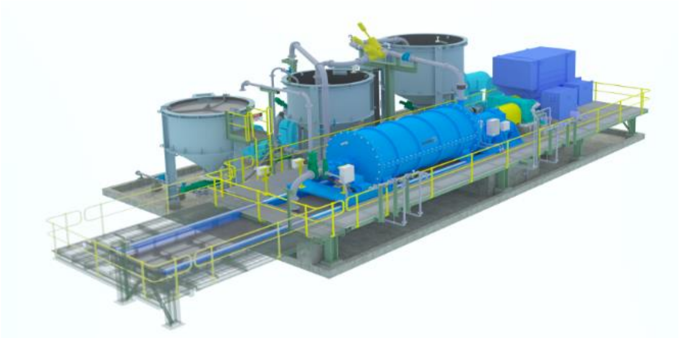
Figure 4 IsaMill™ Fine Grinding Plant
