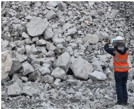
Figure 2: Manual fragmentation analysis using a device with 3D capabilities. Source: Gustavo Huerta Valer.
