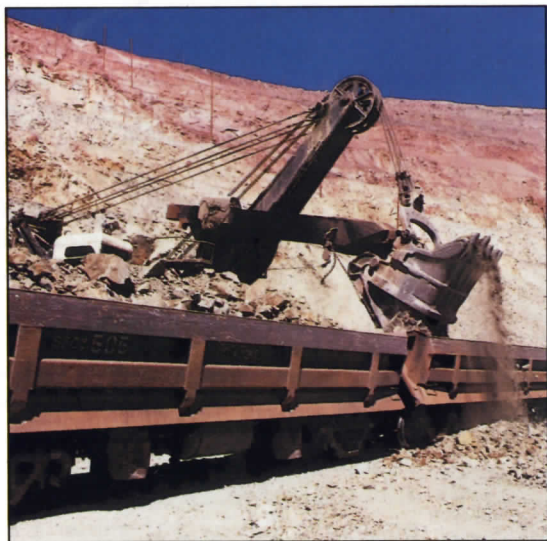
Pala cargando mineral en ferrocarril - Southern Peru Limited
