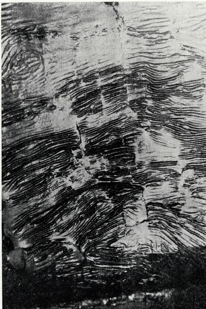
FIG. 1.—Structures produced in decomposed coating of cinema screen
