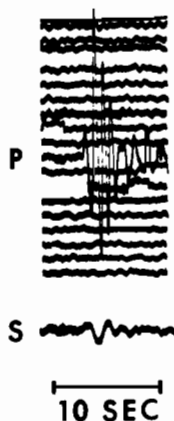
Figure 4B. Recording at Fiji station Vunikawa for earthquake at 208-km depth and 5.7° epicentral distance (after Oliver and Isacks, 1967). Note the almost complete attenuation of the S-wave arrival relative to the P-waves.
