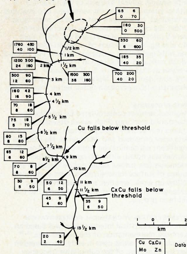
Within and at lower (downstream) end of deposit: Cu > 27, Cx Cu > 47
