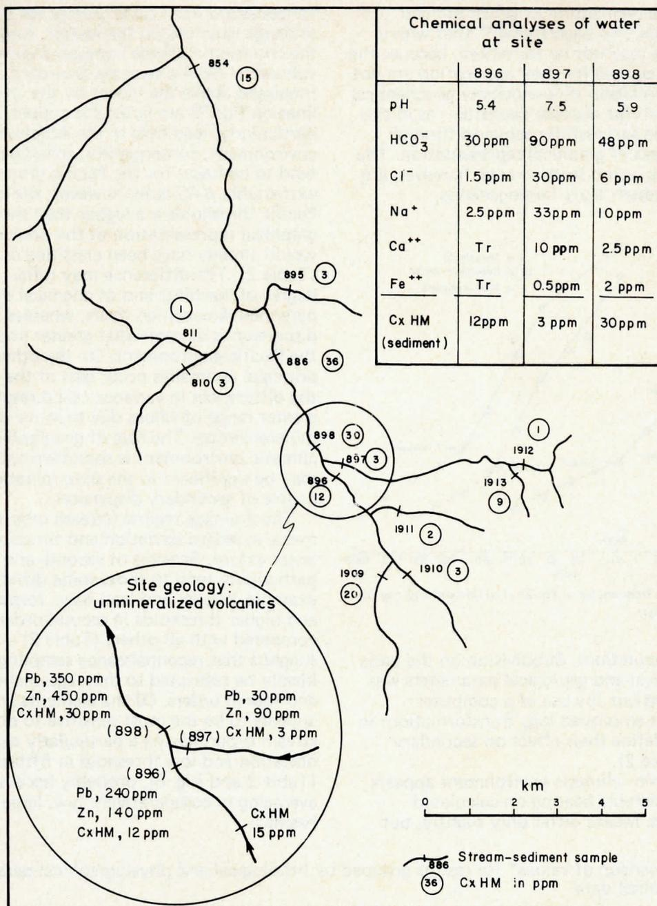
Fig. 5 Example of effect of pH on metal precipitation and anomaly intensity
