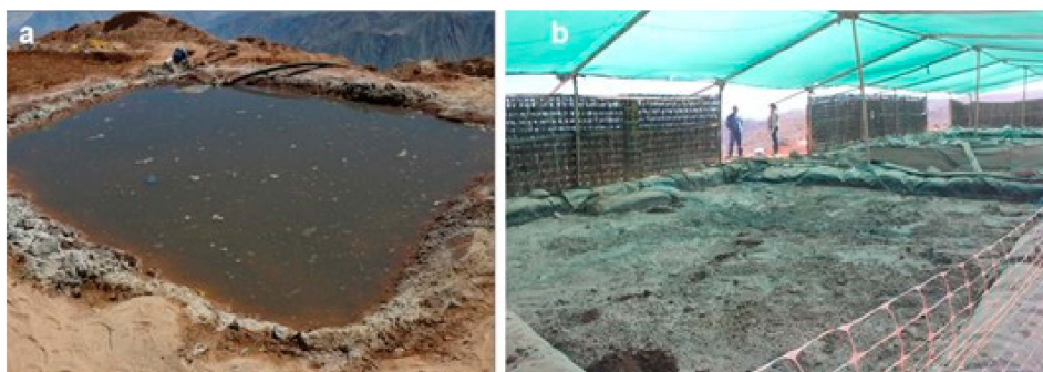
Figure 5. Cyanidation ponds. (a) San Cristobal, image from 2010, (b) In San Luis, the ponds are covered.
