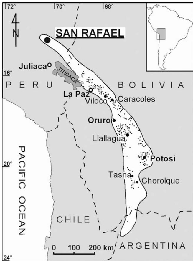
**Fig. 1** Location of the San Rafael Sn–Cu deposit in the Central Andean tin belt (outline and dots representing the deposits are modified after Lehmann 1979; Claire and Minaya 1979)
