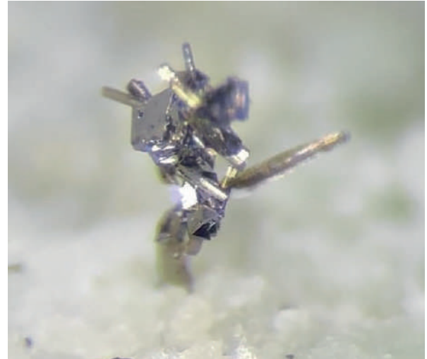
Fig 6. Crystals of siegenite-violarite over millerite needles in a veinlet of Mn-Fe-Ca-Mg carbonate. The carbonate has been attacked with \text{H}_3\text{PO}_4 to reveal the crystal shapes. Image width: 1 mm.
