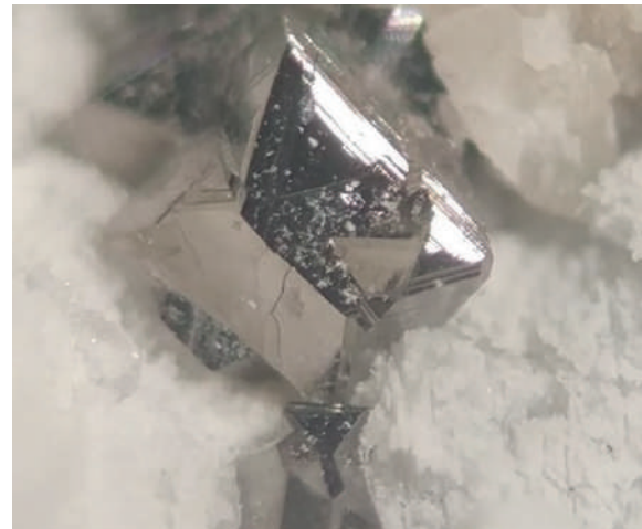
Fig. 7. Twinned (spinel law twin) crystal of siegenite-violarite in a veinlet of Mn-Fe-Ca-Mg carbonate. The carbonate has been attacked with \text{H}_3\text{PO}_4 in order to reveal the crystalline shape. Image width: 1.5 mm.
