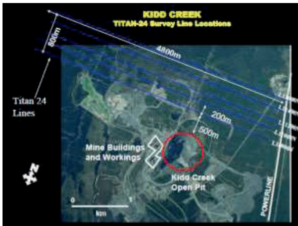
Figure 5. Survey lines near mine and power lines
