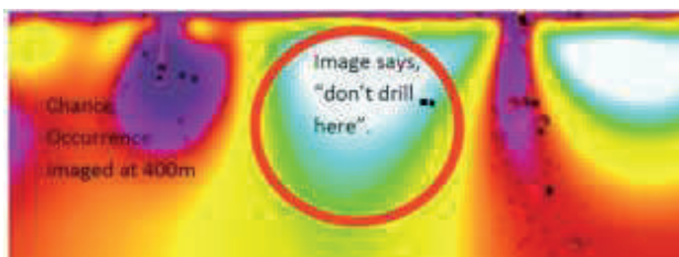
Figure 6 Resistivity section, shown to > 700m depth. Blue/ white regions represent resistive rock, warm colors represent increased conductivity
