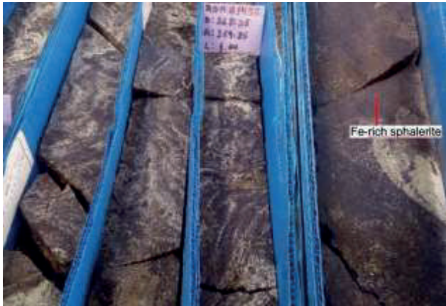
Fig. 4 Massive ore consisting mainly of Fe-rich sphalerite typical for the richest portions of the Puagjanca pipe. Drill core width: 6.3 cm
