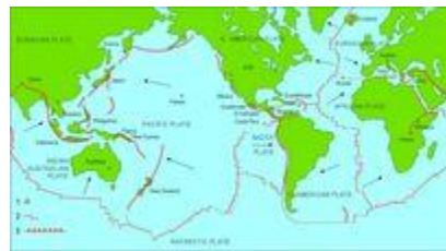
Figure 5: World pattern of plates, oceanic ridges, oceanic trenches, subduction zones, and geothermal fields. Arrows show the direction of movement of the plates towards the subduction zones. (1) Geothermal fields producing electricity; (2) mid-oceanic ridges crossed by transform faults (long transversal fractures); (3) subduction zones, where the subducting plate bends downwards and melts in the asthenosphere.
