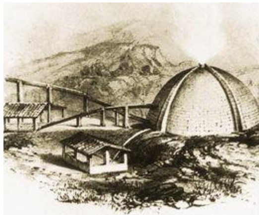
Figure 2: The “covered lagoon” used in the first half of the 19th century in the Larderello area, Italy, to collect the hot boric waters and extract the boric acid.
