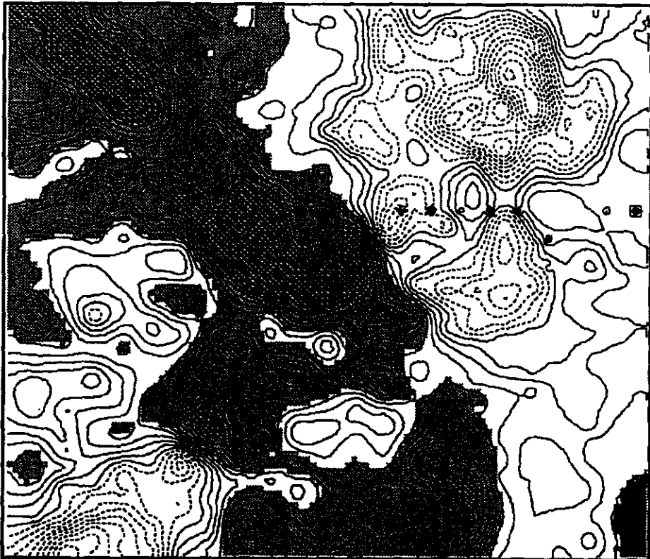
Fig. 3. Kriging map from 1665 Cu-values. Power-law model was used. Solid lines represent relatively high values and dashed lines for relatively low values. The shaded patterns represent the anomalies identified by means of the concentration - area fractal model in a spatial domain (see text for detailed explanation).
