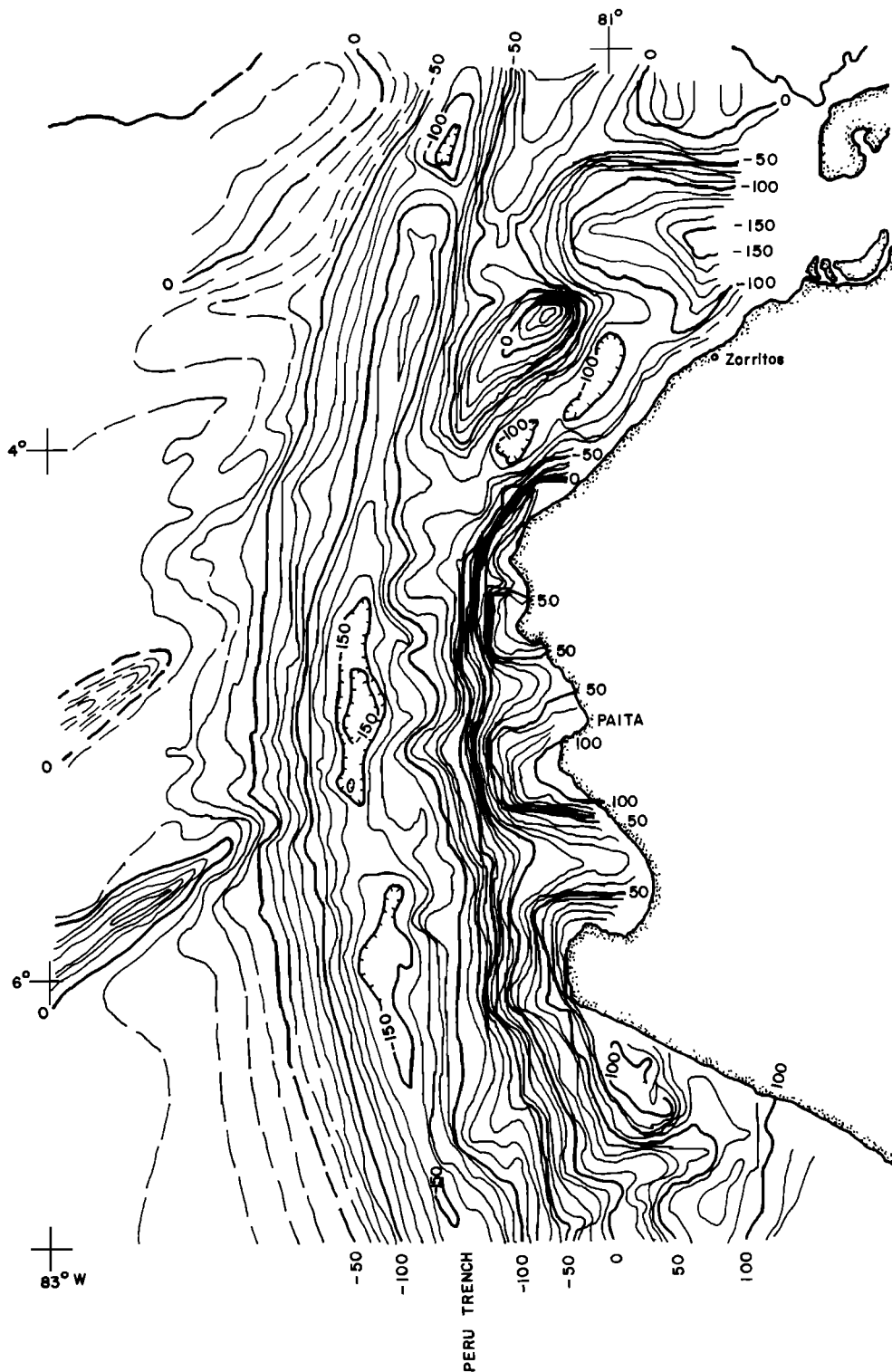
Fig. 5. Detailed gravitational anomaly (free air) map off-shore northwest Peru, 2.5°- 7°S latitudes. The anomalies produced by deep ocean ridges and shelf capes are strong (after Shepherd, 1979).
