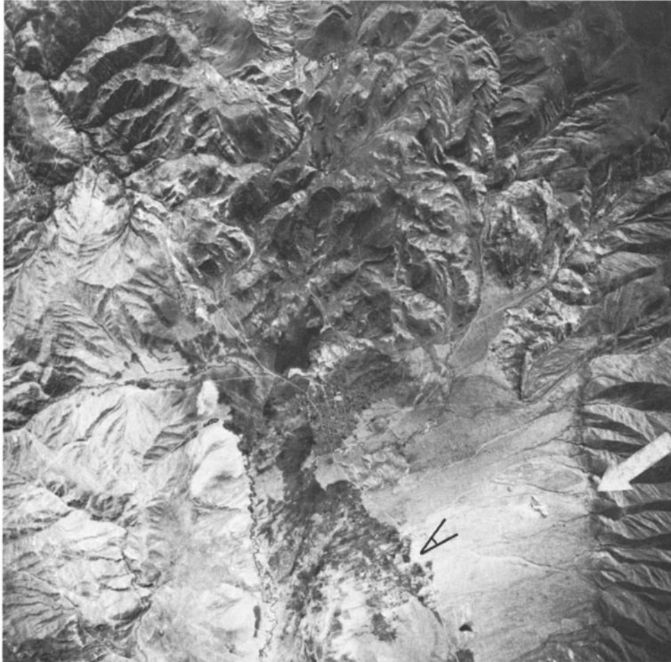
Fig. 13. Aerial photograph of an active normal fault in the Altiplano of southern Peru. Arrow points to the fault scarp. Photo shows an area of approximately 8 by 8 km. The town of Sangarara (-13.95, -71.60) is near the center of the photograph.
