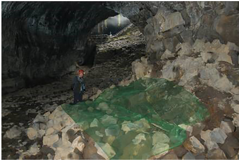
Fig. 3. Monitoring for rockfall using a plastic net in Manjanggul Cave (lava tube) which is located under the traffic road.
