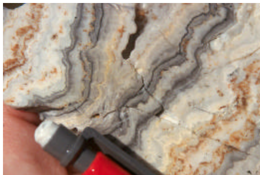
Photo 20. Banded adularia-sericite epithermal gold-silver mineralization showing well developed banded quartz and ginguro ore from Golden Cross.
