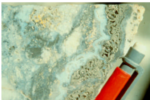
Photo 3. Low temperature quartz-sulphide gold ± copper mineralization from Rawas containing opaline silica and marcasite-pyrite
