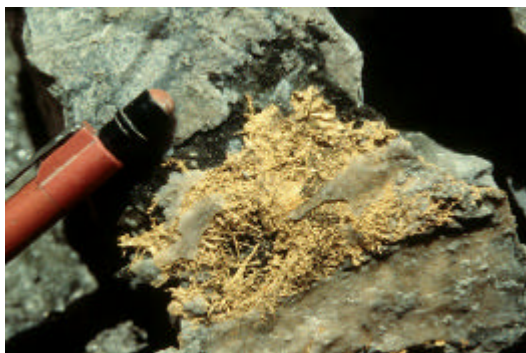
Photo 17. Bonanza epithermal quartz gold-silver mineralization from Porgera Zone VII containing wire gold, quartz and roscoelite.
