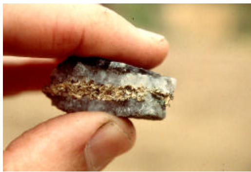
Photo 18. Bonanza gold grade epithermal quartz gold-silver style mineralization comprising gold fill of an open quartz vein, Edie Creek.
