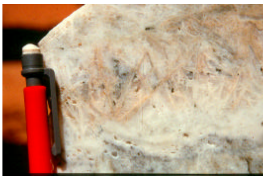
Photo 21. Adularia-sericite epithermal gold-silver mineralization showing well developed quartz pseudomorphing platy calcite from Vera Nancy.
