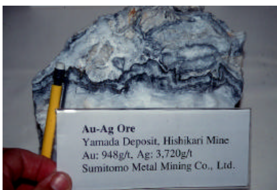
Photo 23. High grade (948 g/t Au, 3720 g/t Ag) adularia-sericite epithermal gold-silver vein with abundant mineralised ginguro material, Hishikari.
