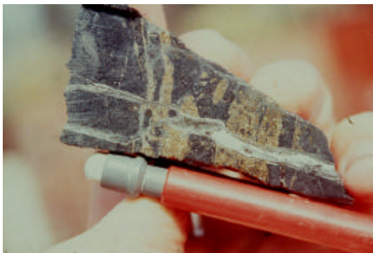
Photo 13. Carbonate-base metal gold vein cuts quartz-sulphide gold \pm copper mineralization, Mt Kare
