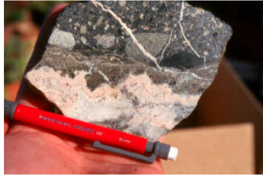
Photo 12. Carbonate-base metal gold mineralization postdates diatreme breccia from Upper Ridges, Wau. Note the paragenetic sequence evident as breccia -> sulphides -> carbonate.
