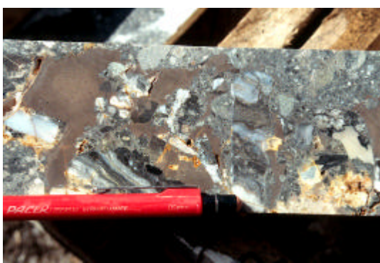
Photo 24. Toka Tindung eruption breccia with sinter and wood fragments in a strongly silicified matrix
