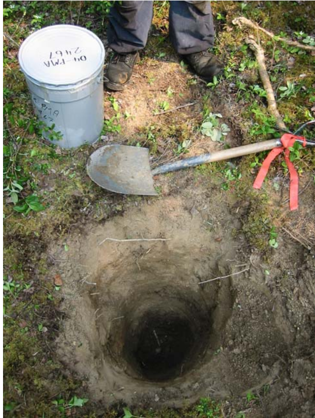
Figure 3. Example of sample collected in a hand-dug pit.
