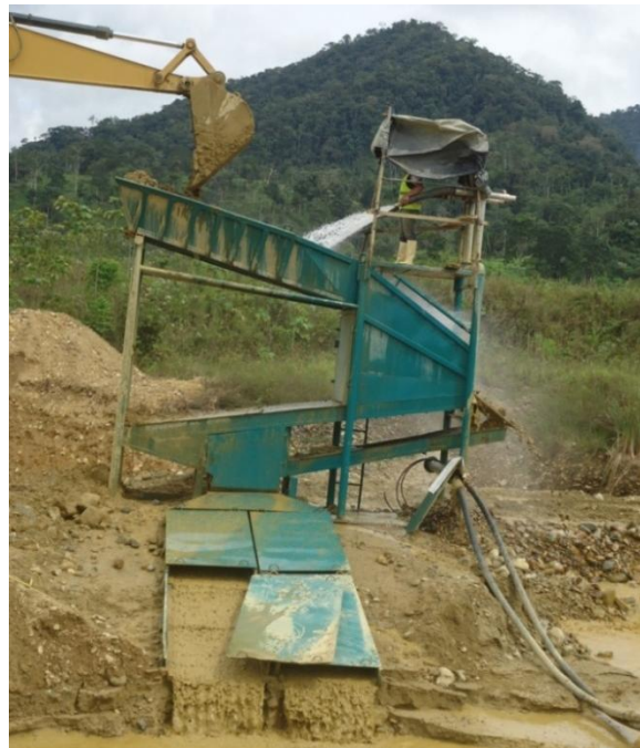
Figure 6. Gravity concentrator in sluice boxes
