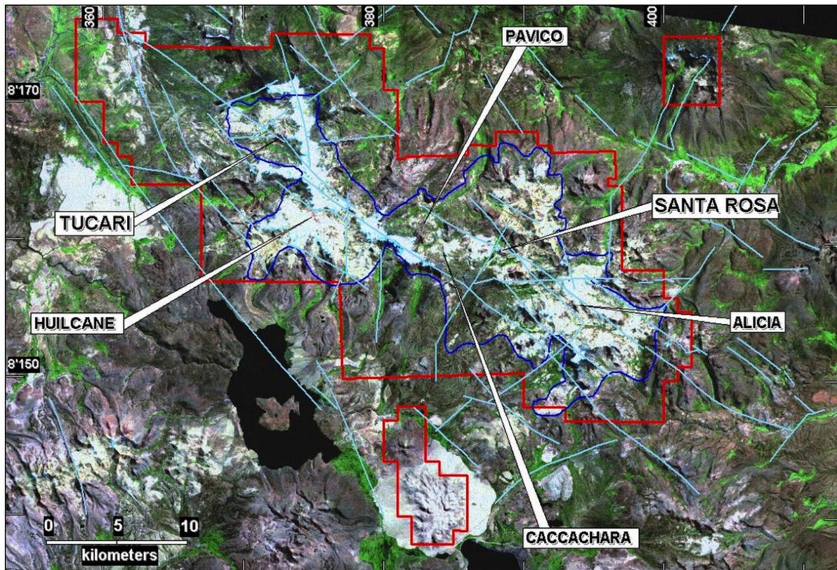
Figure 3. Landsat TM image: Outline of alteration (dark blue), principal structures (light blue) and principal centers of mineralization within the Aruntani district. The old silver-base metal mines Pavico and Caccachara are shown.
