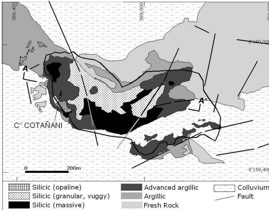
Figure 4. Santa Rosa deposit, plan map: Types of alteration, and outline of final pit design.
