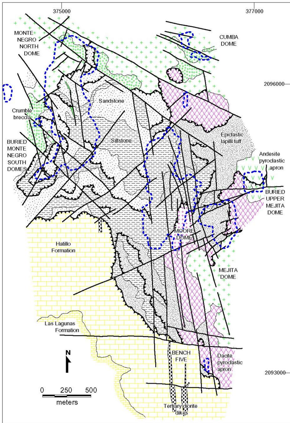
Fig. 2. Geologic map of the Pueblo Viejo district showing the location of volcanic domes and pit outlines (heavy dotted line). See Table 2 for an explanation of rock units. Strike and dip symbols are omitted for clarity; sedimentary units are subhorizontal. See Figure 3 for a detailed geologic map of the Moore deposit.
