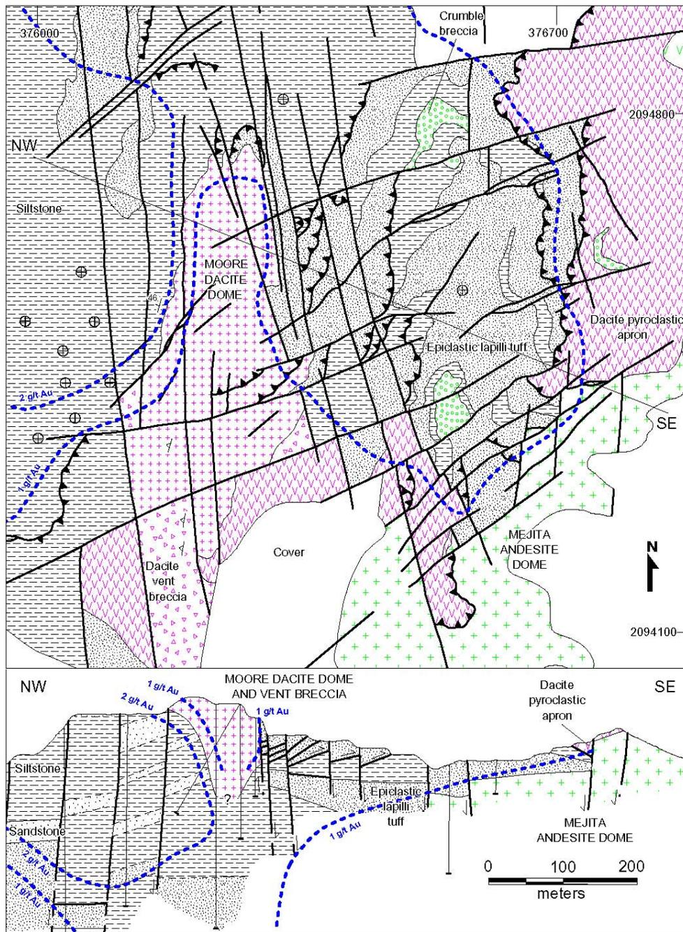
Fig. 3. Geologic map and cross section of the Moore deposit, Pueblo Viejo district. There is no vertical exaggeration. Rock units too thin to be shown clearly on the section are omitted. Drill hole locations are plotted on the section. Grade contours are shown as heavy dotted lines.
