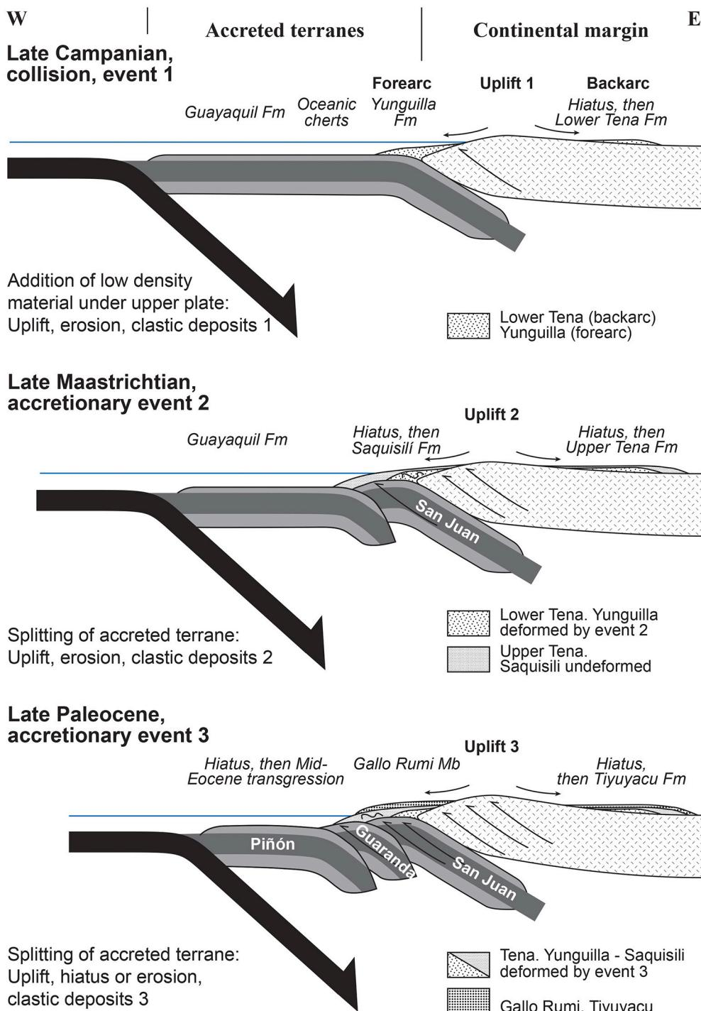
**Fig. 13.** Model for the accretion of oceanic terranes, accounting for the uplift, deformation, hiatuses and deposition observed in the forearc (accreted terranes) and backarc (Oriente Basin) areas of the Ecuadorian margin. The first accretionary event led to the end of the San Lorenzo island arc activity located on the accreted oceanic plateau. Arc volcanism resumed in latest Maastrichtian-Paleocene times, after accretionary event 2, on the continental margin.
