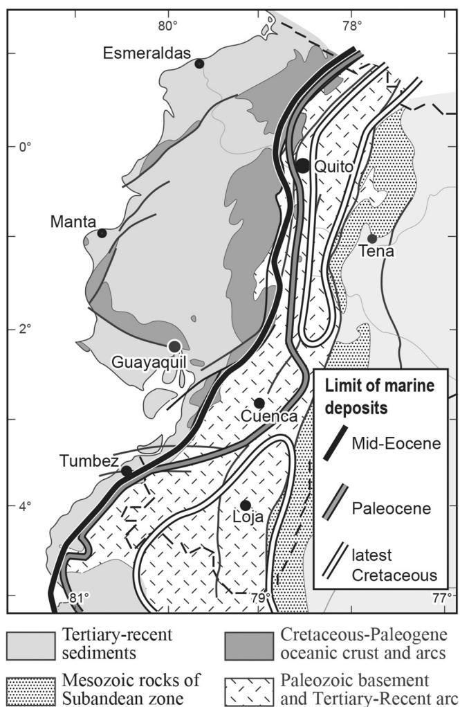
**Fig. 7.** Evolution of the marine shoreline from Maastrichtian to Late Eocene times (from Toro and Jaillard, 2005). Marine environment persisted on the oceanic terranes during this whole time-span, whereas most of the forearc zones and the Oriente Basin became emergent in latest Cretaceous and Paleocene times, respectively.
