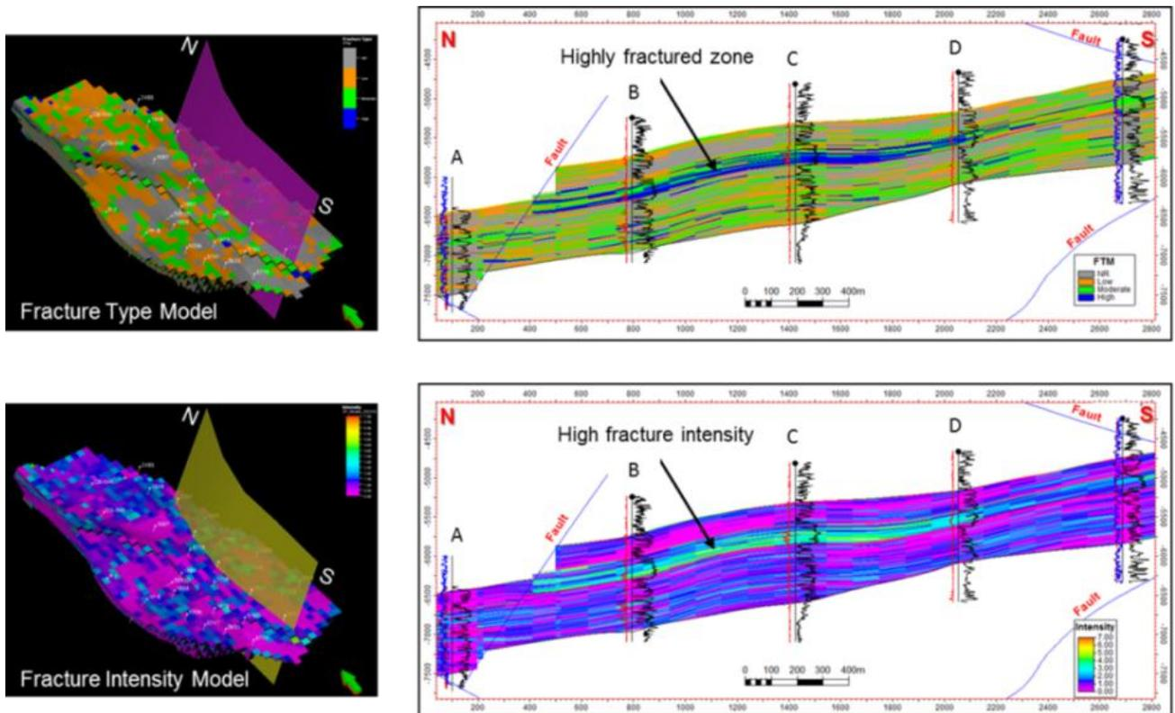
**Figure 3.** Rock or fracture type and fracture intensity models obtained from the integration of well logs. Observe the intervals that fracture more easily characterized by rock type high and a high fracture intensity values.
