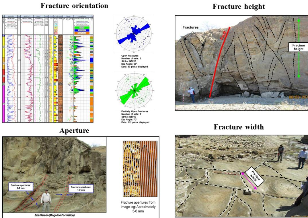
Figure 4. Information used to characterize natural fracture networks.
