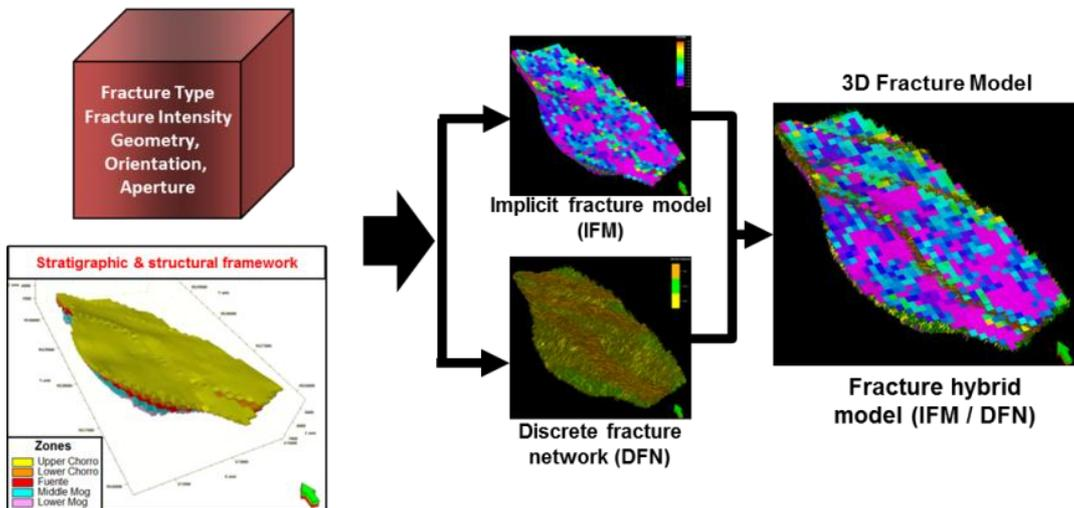
Figure 5. Attributes of fractures and structural framework of the reservoir were integrated to obtain the 3D fracture model consisting of the discrete fracture network and implicit fracture model.
