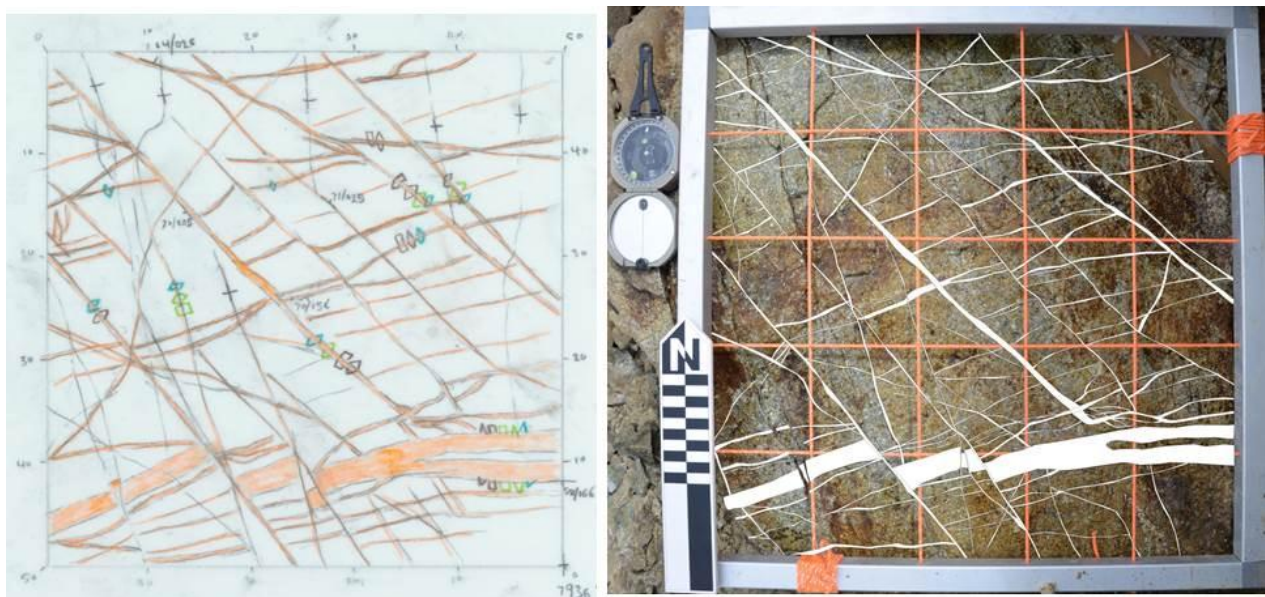
Figure 1. Example of field map, mapping grid and digitized veins from within the Ferrobamba deposit
