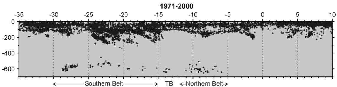
**Figure 5-** Longitudinal NS profile beneath the Andean Region showing several important seismotectonic features of the Nazca subducted slab. The Central Andes region is located between 15° and 18° S.
