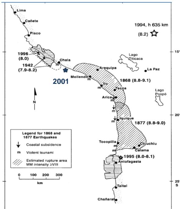
**Figure 1-** Seismic gap in the Peru/Chile border region. Isoseismals VIII MM represents the rupture of the earthquakes. Modified from Spence *et al.* (1999)
