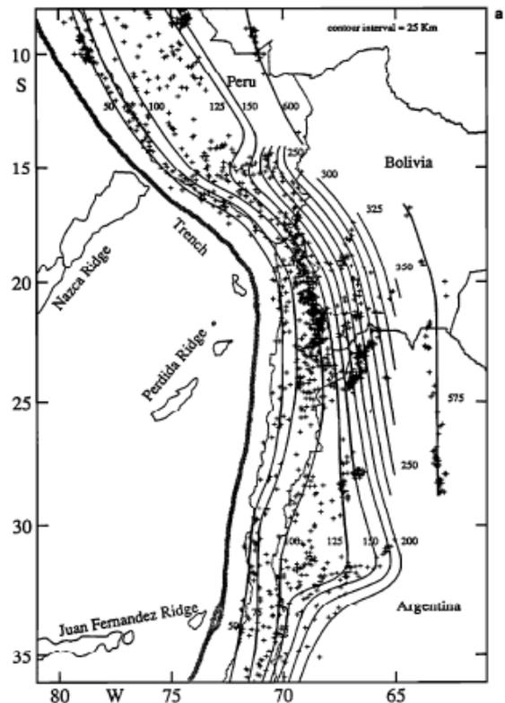
**Figure 2-** Contours map of Nazca slab showing some seismotectonic features beneath the Andean region. Cahill & Isacks (1992)
