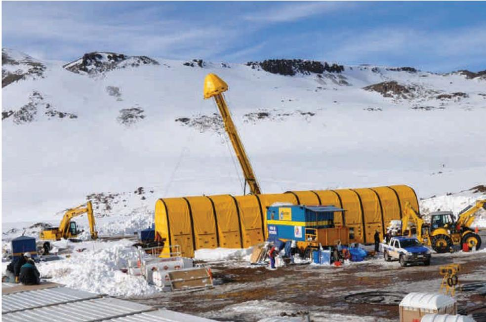
*Figure 4. Coring rig drilling an inclined hole during winter conditions on Magma’s Laguna del Maule exploitation concession in Chile (photo by Frank Baumann).*
