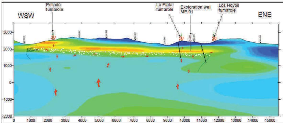
Figure 3. 2D resistivity model of Magma's Mariposa reservoir, central Chile, from an MT survey. Dashed line represents the 200°C isotherm inferred from the data and the likely top of the reservoir below a clay cap.
