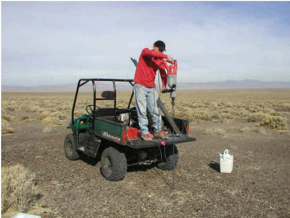
Figure 2. Insertion of 2-meter-long hollow steel pipe into the ground using an electric hammer and portable generator mounted on an all-terrain vehicle (ATV). Temperatures at a 2-meter depth can be measured by inserting a digital resistance temperature device down the middle of the pipe.
