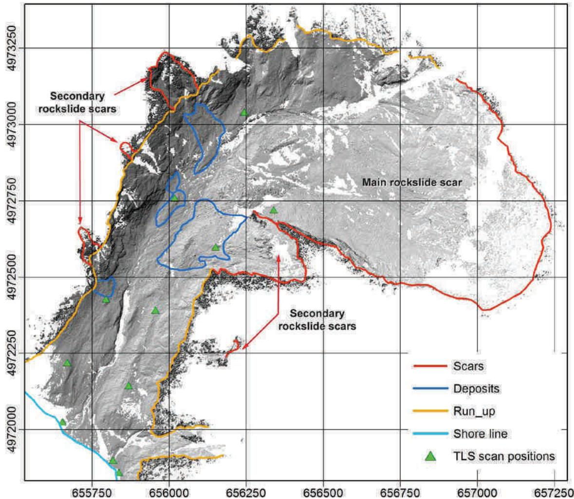
Figure 3. Hillshade of the HR-DEM created from the TLS point clouds of the Punta Cola rockslide scar and the rock avalanche deposits. The main morphological features of the rock avalanche and the TLS scan positions are shown (coordinates in UTM 18S).
