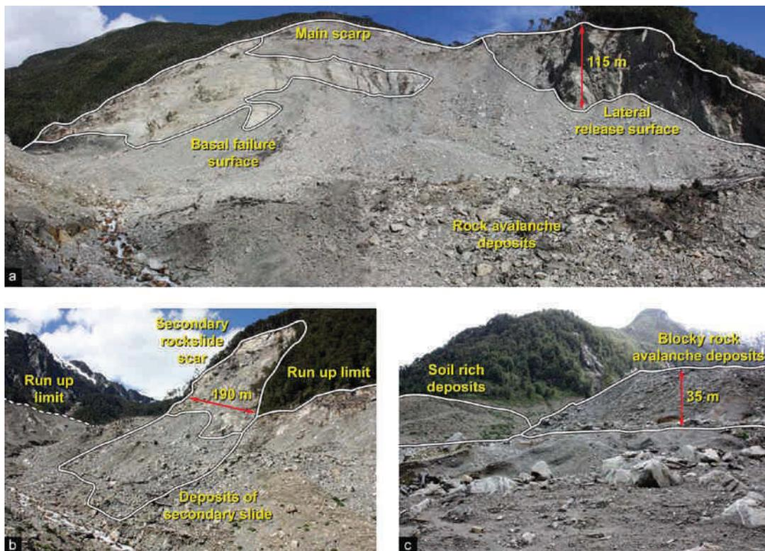
Figure 2: Photographs of the Punta Cola rock avalanche: a) panorama of the rockslide scar displaying the outcropping basal failure surface and the 115 m high lateral release surface. A branch of the LOFZ passes across the lateral release surface and the head scarp; b) secondary rockslide scar, associated deposits and run up limits of the main rock avalanche on the right valley side; c) steep rock avalanche deposits with different compositions (blocky vs. soil rich).
