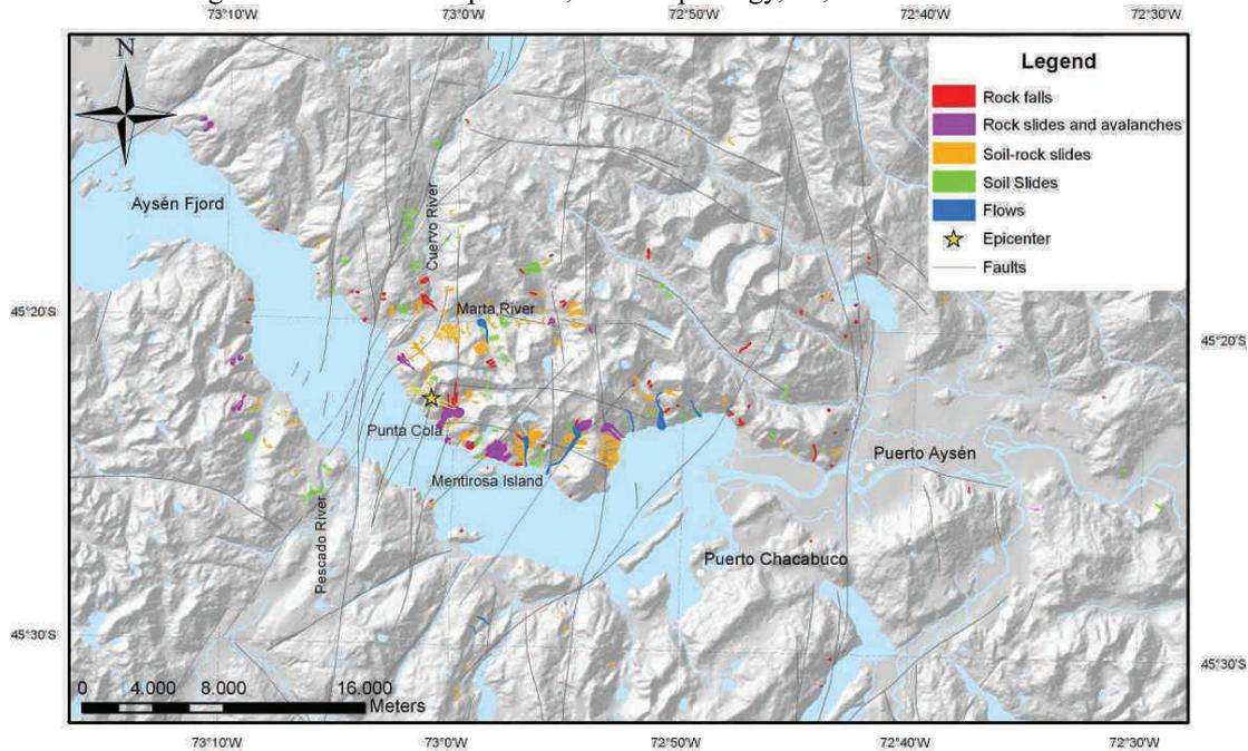
Figure 1. Distribution of landslides triggered by the 21 April 2007 Aysén earthquake [Sepúlveda et al., 2010]. The Punta Cola rock avalanche occurred in immediate vicinity to the epicentre.
