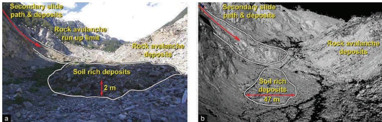
Figure 4. a) Lobate soil rich landslide deposits in the run out area of the Punta Cola rock avalanche attest that scouring by the rock avalanche along valley flanks caused secondary landslides contributing significantly to the total landslide volume; b) terrestrial laser scanner point cloud with similar view as the photograph reveals the morphology of the different deposits, including the soil rich lobe deposited onto the main rock avalanche deposits.
