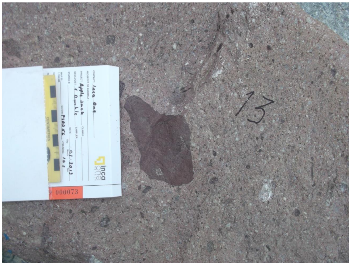
Figure 20 Sample 13 iron oxide altered coarse clastic tuff
