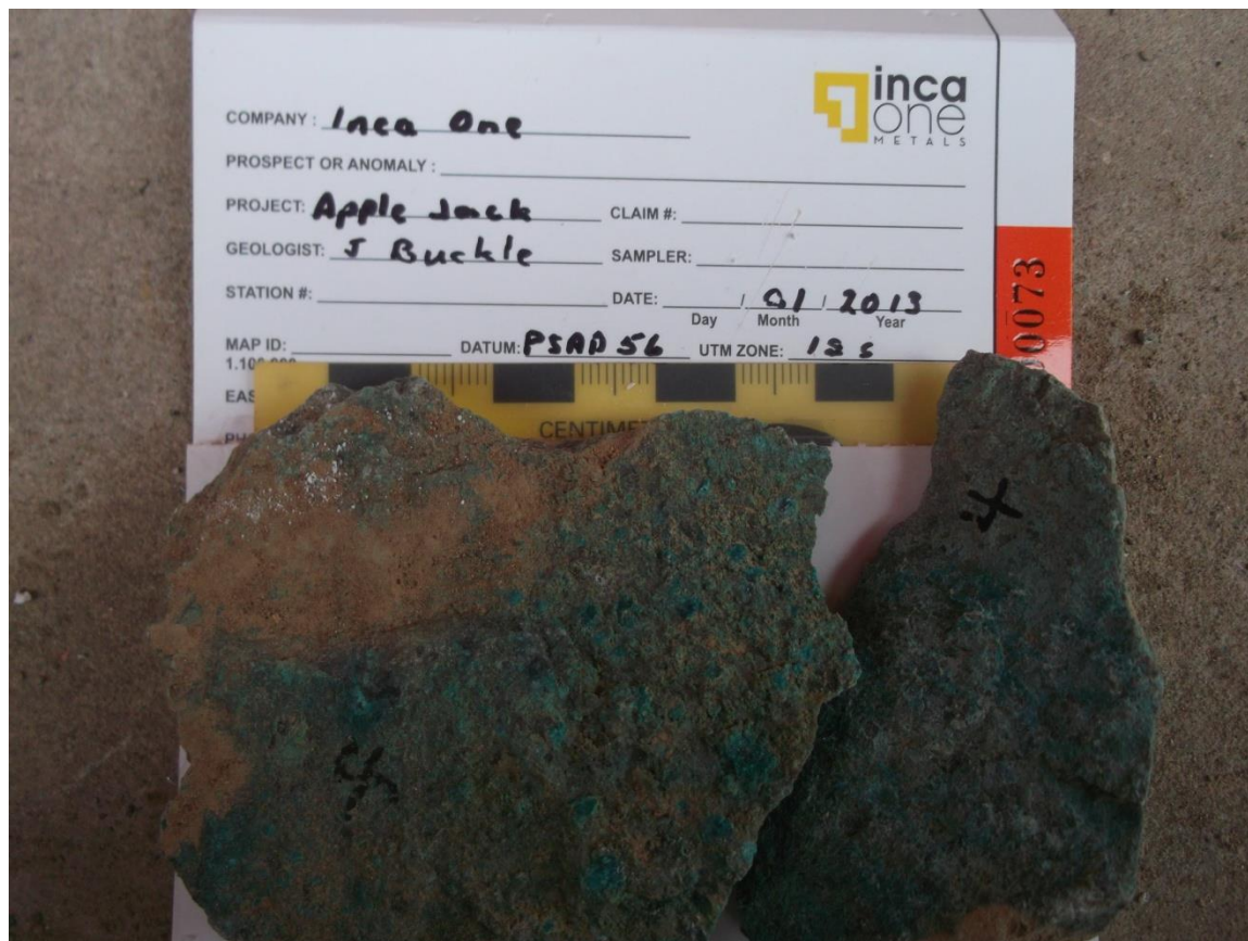
Figure 11 Hand sample 4 replacement copper oxides malacite/asurite in tuff
