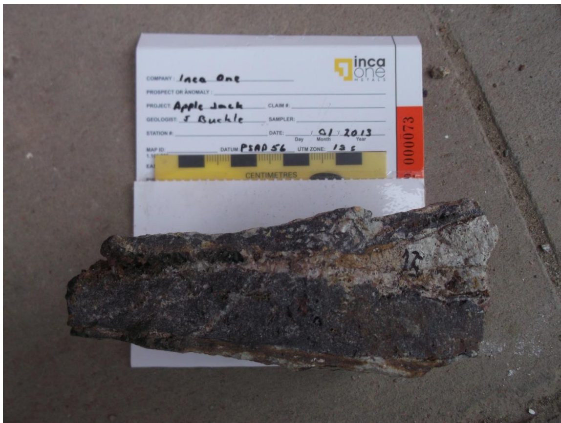
Figure 22 Hand sample 15 silicified hematite quartz bedded tuff
