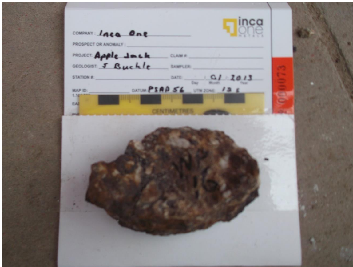
Figure 23 Hand sample 16 iron oxidized matrix of quartz vein breccia
