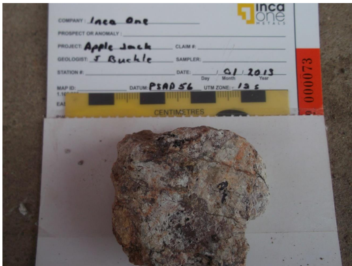
Figure 16 Hand sample 9 silicified tuff with vitreous quartz eyes
