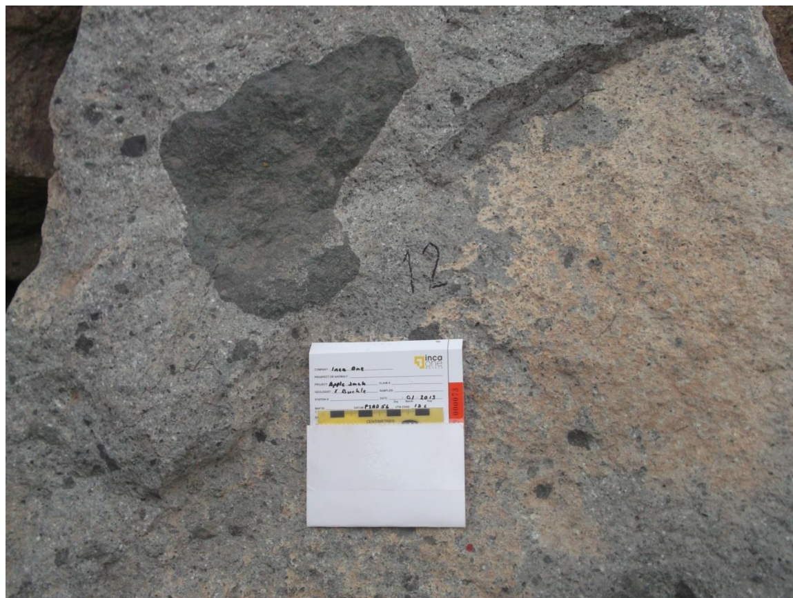
Figure 19 Sample 12 coarse clastic andesite-dacite tuff with clasts to 0.5 meters
