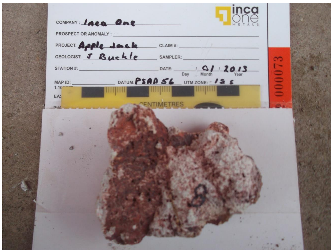
Figure 15 Hand sample 8 kaolinite-jarosite altered quartz vein
