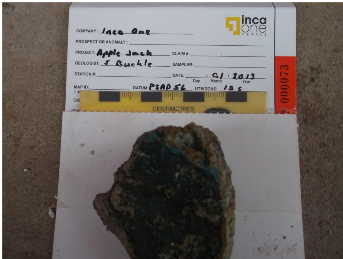
Figure 17 Hand sample 10 malachite-azurite-specular hematite replacement in silicic tuff
