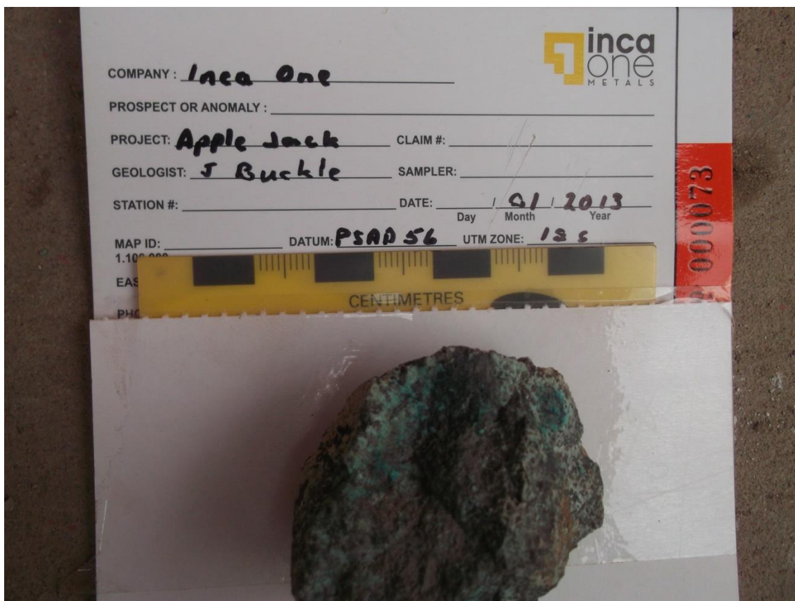
Figure 21 Hand sample 14 copper and iron oxide replacement in tuff
