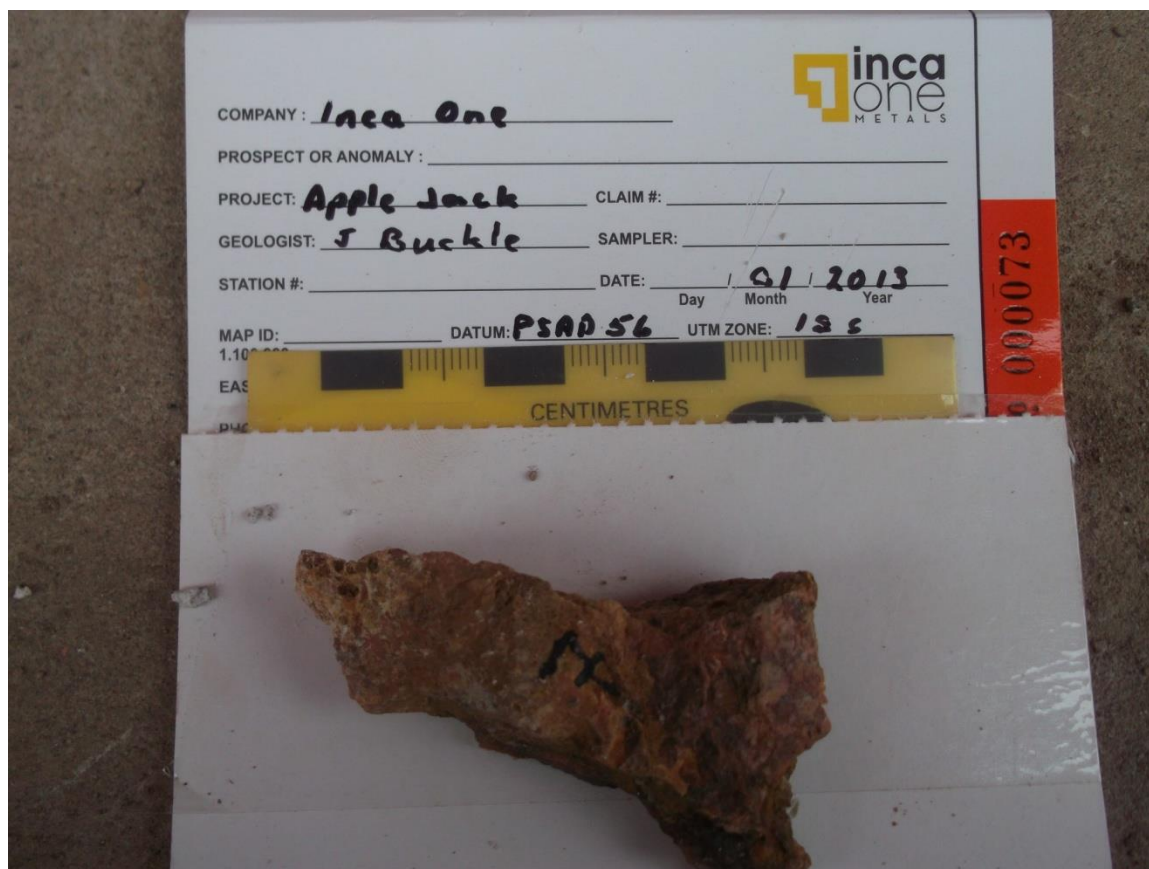
Figure 14 Hand sample 7 earthy iron oxidized mineralized vuggy quartz after iron sulphides
