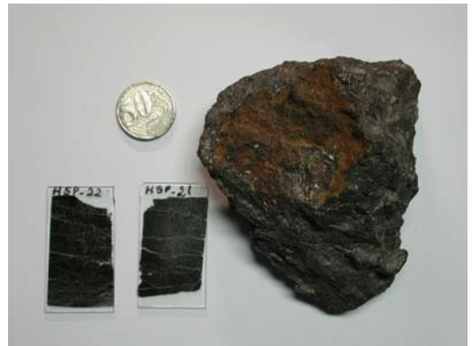
Figure 3- Photography of massive podiform chromitite from Morro Feio ultramafic body, Brasília belt, (Goiás State).
