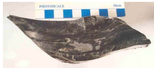
Figure 2. Rock fragment from an anastomose fracture system controlled by foliation overprinting (scale marks are cm) (Chariot gold mine, NT, sample courtesy of Joel Anders).
