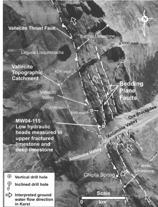
Figure 5. Drilling Investigation – Antamina Valley
