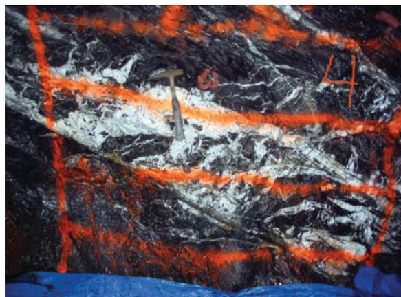
3 Panel sample preparation at the Liphichi gold project. One-hundred kilogram samples taken for metallurgical testing and grade verification
