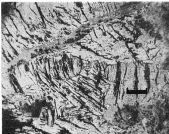
FIG. 10—Granular pyrolusite, a probably supergene alteration from manganite, showing parallel shrinkage cracks. Geothite vein (grey). Bar is 0.02 mm.
