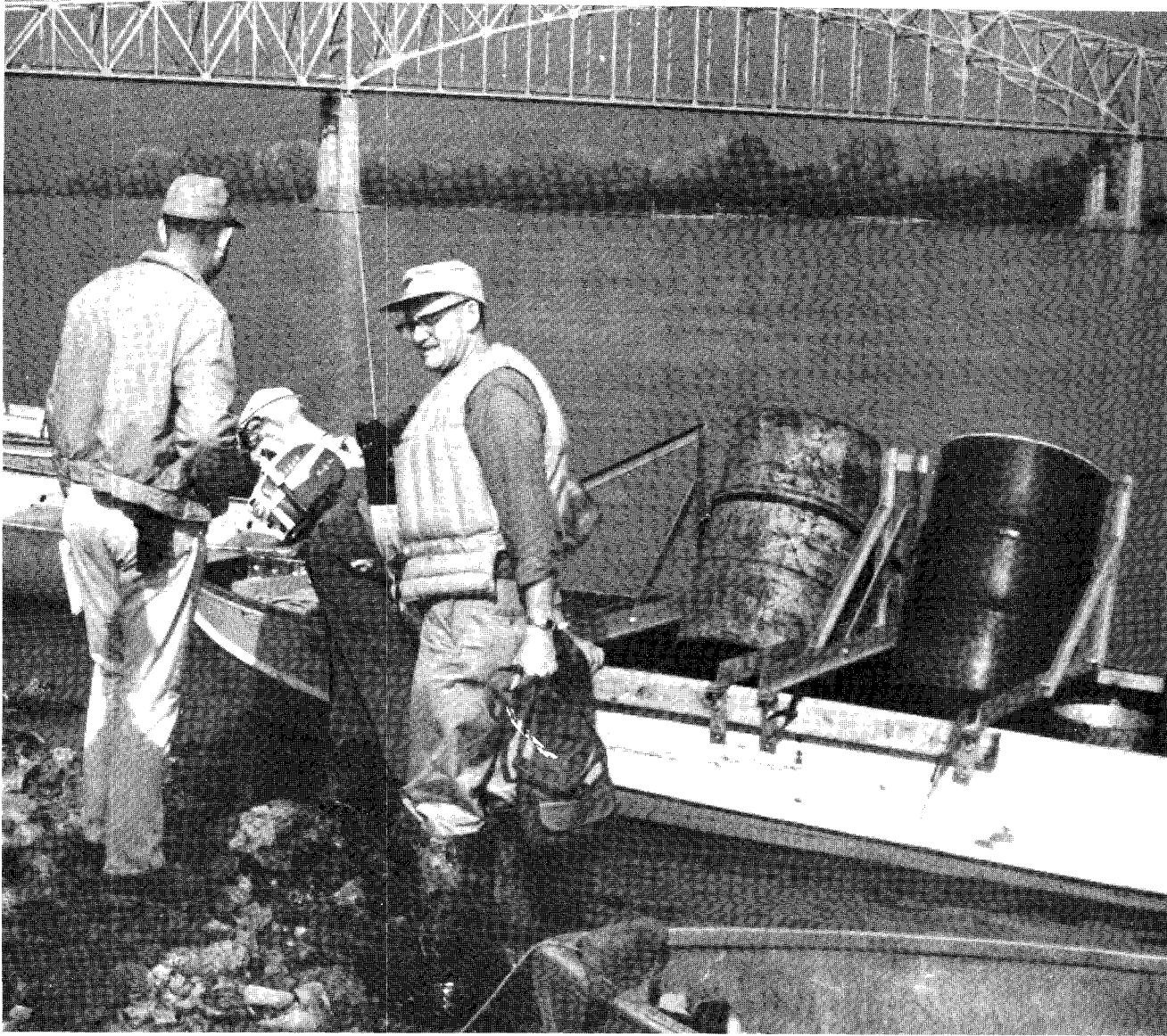
Figure 4.—Special boat-mounted apparatus for making a line injection of a large dosage of dye. (Photograph by Missouri district of U.S. Geological Survey.)
